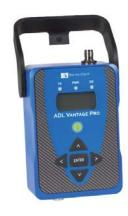
Radio modems from Pacific Crest provide wireless data links for RTK positioning and remote sensing. These broad spectrum transceivers offer up to 35 Watts of power and over-the-air link rates as high as 19,200 Baud. Pacific Crest is the leading provider of high-performance data links for the Geomatics industry based on the acceptance of its communications protocols as the standard for RTK surveying.
