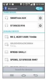
*Note:* The rover is identified by XDLROVER, followed by the radio's unique serial number. This ensures that you always select the right unit when there are multiple units within Bluetooth range.
