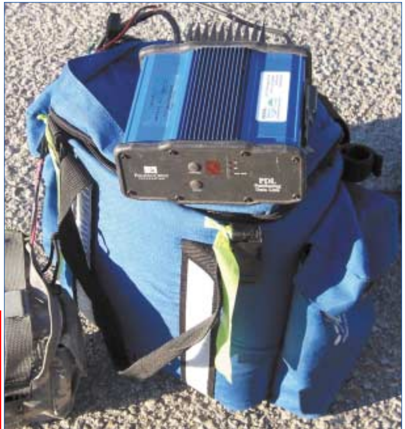
Fig 1 – PDLHPB 2/35 watt base radio - note external antenna cable and external battery (in camo pack). Data & power use same Lemo connector, antenna uses BNC connector.
